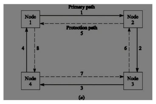
Ex: Total capacity OC-12 may be divided to four OC-3 streams, the OC-3 is called a path here
