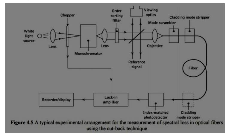
The fiber is also usually put through a cladding mode stripper, which may consist of an S-shaped groove cut in the Teflon and filled with glycerine. This device removes light launched into the fiber cladding through radiation into the index-matched (or slightly higher refractive index) glycerine. A mode stripper can also be included at the fiber output end to remove any optical power which is scattered from the core into the
