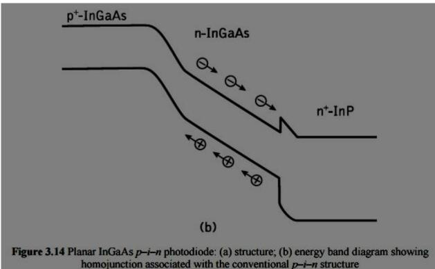
The top entry\* device shown in Figure 3.14(a) is the simplest structure, with the light being introduced through the upper p+-layer. However, a drawback with this structure is
