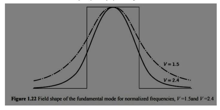
As may be expected, considering the discussion in Section 2.4.1, it has the form of a Bessel function  $(J_0(r))$  in the core region matched to a modified Bessel function  $(K_0(r))$  in the cladding. Depending on the value of the normalized frequency, a significant proportion of the modal power is propagated in the cladding region, as mentioned earlier. Hence, even at the cutoff value (i.e.  $V_c$ ) only about 80% of the power propagates within the fiber core.
