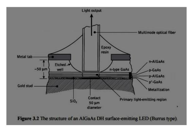
However, the power coupled into the fiber is also dependent on many other factors including the distance and alignment between the emission area and the fiber, the SLED emission pattern and the medium between the emitting area and the fiber. For instance, the addition of epoxy resin in the etched well tends to reduce the refractive index mismatch and increase the external power efficiency of the device. Hence, DH surface emitters often give more coupled optical power than predicted by Eq. (3.1).
