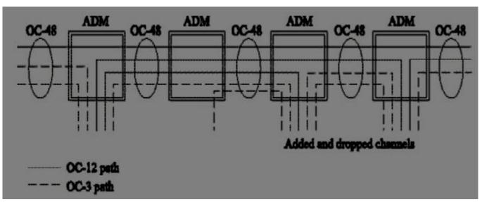
SONET ADM is a fully synchronous, byte oriented device, that can be used add/drop OC sub-channels within an OC-*N* signal
