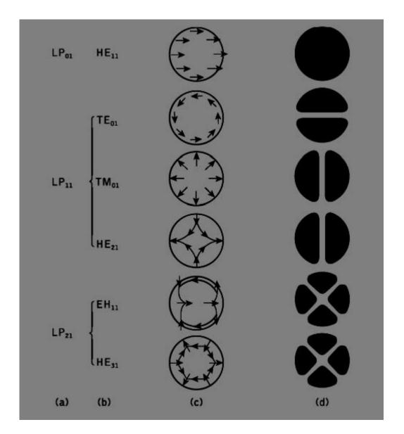
Figure 1.11 The electric field configurations for the three lowest LP modes illustrated in terms of their constituent exact modes: (a) LP mode designations; (b) exact mode designations; (c) electric field distribution of the exact modes; (d) intensity distribution of Ex for the exact modes indicating the electric field intensity profile for the corresponding LP modes
