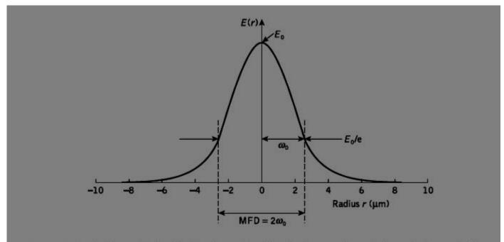
Figure 1.19 Field amplitude distribution E(r) of the fundamental mode in a single-mode fiber illustrating the mode-field diameter (MFD) and spot size ( $\omega_{\square}$ )
