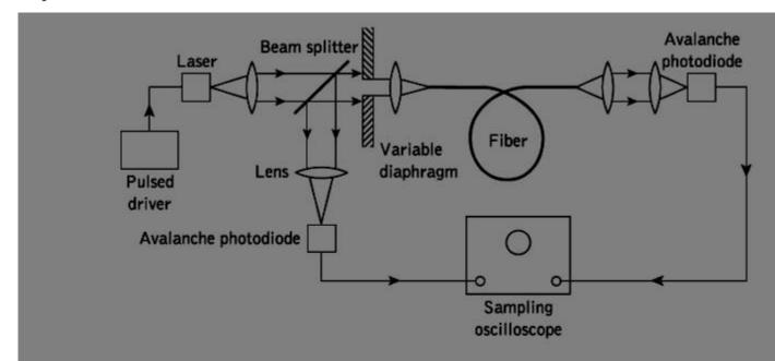
Figure 4.9 Experimental arrangement for making multimode fiber dispersion measurements in the timdomain.
