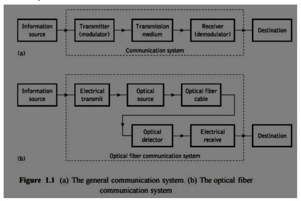
The optical carrier may be modulated using either an analog or digital information signal. In the system shown in Figure 1.1(b) analog modulation involves the variation of the light emitted from the optical source in a continuous manner. With digital modulation, however, discrete changes in the light intensity are obtained (i.e. on–off
