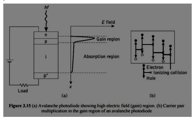
This process is known as impact ionization and is the phenomenon that leads to avalanche breakdown in ordinary reverse-biased diodes. It often requires high reverse
