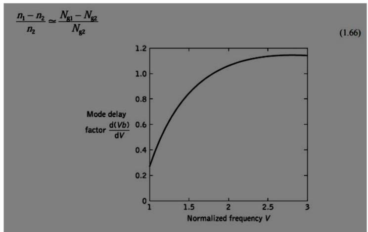
Figure 1.21 The mode delay factor (d(Vb)/dV) for the fundamental mode in a step index fiber shown as a function of normalized frequency (V)
