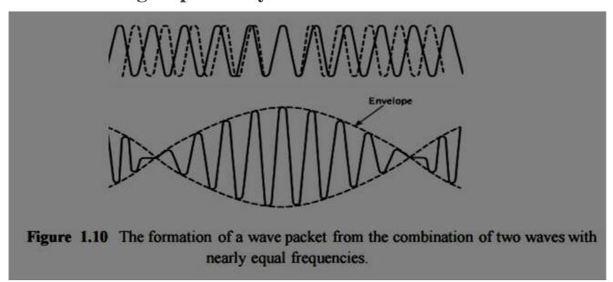
The envelope of the wave package or group of waves travels at a group velocity vg With in all electromagnetic waves, whether plane or otherwise, there are points of constant phase. For plane waves these constant phase points form a surface which is referred to as a wavefront. As a monochromatic lightwave propagates along a waveguide in the z direction these points of constant phase travel at a phase velocity vp given by
