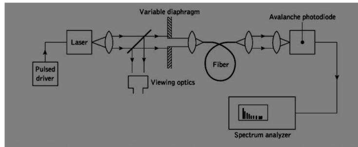
Figure 4.10 Experimental setup for making fiber dispersion measurements in the frequency domain using a pulsed laser source
