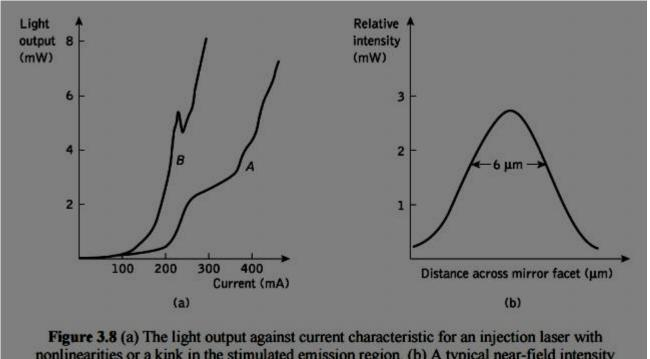
nonlinearities or a kink in the stimulated emission region. (b) A typical near-field intensity distribution (pattern) in the plane of the junction for an injection laser
