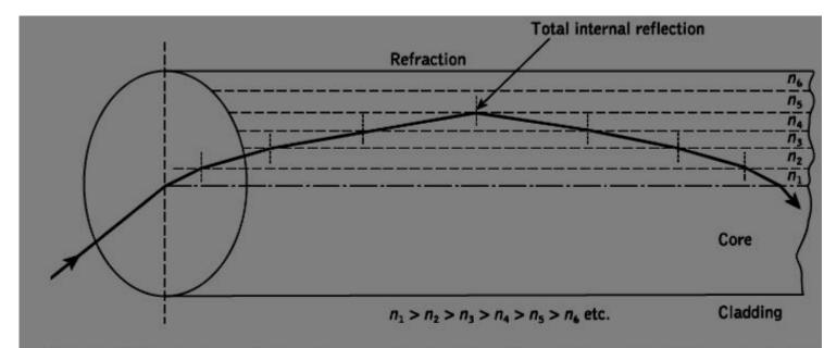
Figure 1.17 An expanded ray diagram showing refraction at the various high to low index interfaces within a graded index fiber, giving an overall curved ray path into the outer regions of the core.
