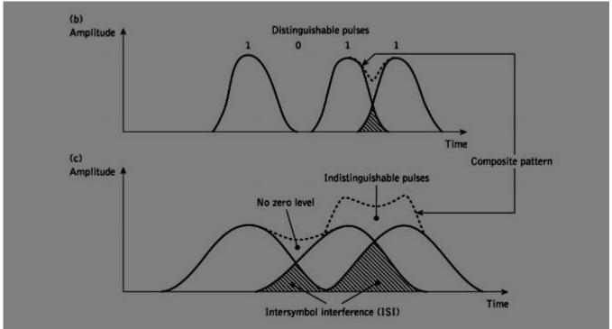
Figure 2.7 An illustration using the digital bit pattern 1011 of the broadening of light pulses as they are transmitted along a fiber: (a) fiber input; (b) fiber output at a distance L1; (c) fiber output at a distance L2 > L1
