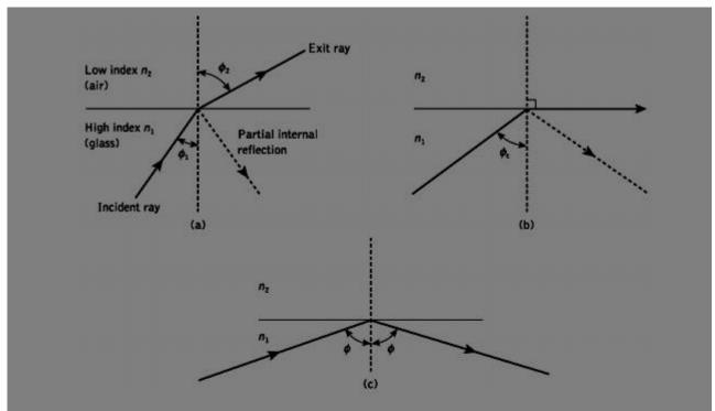
Figure 1.2 Light rays incident on a high to low refractive index interface (e.g. glass air): (a) refraction; (b) the limiting case of refraction showing the critical ray at an angle φ<sub>C</sub> (c) total internal reflection where φ>φ<sub>C</sub>
