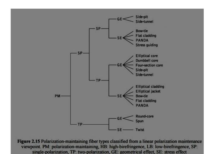
The various types of PM fiber, classified in terms of their linear polarization maintenance, are shown in Figure 2.16
