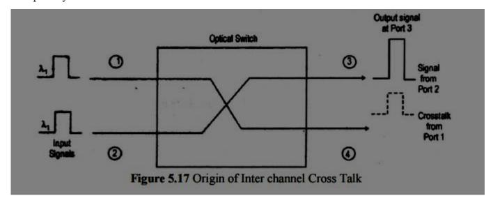
Two independent signals, each at a wavelength  $\lambda 1$ , enter an optical switch.
