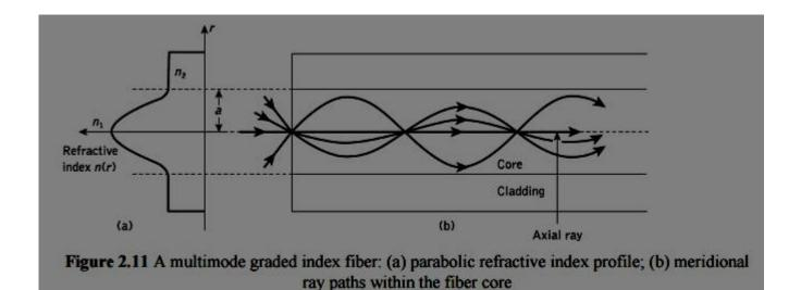
Hence there is an equalization of the transmission times of the various trajectories towards the transmission time of the axial ray which travels exclusively in the high-index region at the core axis, and at the slowest speed. As these various ray paths may be considered to represent the different modes propagating in the fiber, then the graded profile reduces the disparity in the mode transit times.
