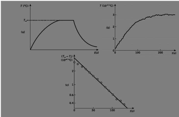
Figure 4.7 (a) A typical heating and cooling curve for a glass fiber sample. (b) A heating curve. (c) The corresponding plot of  $(T\infty - Tt)$  against time for a sample glass rod
