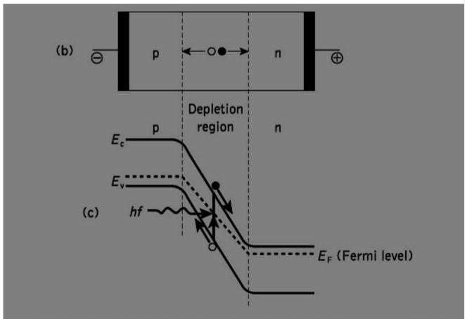
Figure 3.11 Operation of the *p-n* photodiode: (a) photogeneration of an electron-hole pair in an intrinsic semiconductor; (b) the structure of the reverse-biased *p-n* junction illustrating carrier drift in the depletion region; (c) the energy band diagram of the reverse-biased *p-n* junction showing photogeneration and the subsequent separation of an electron-hole pair
