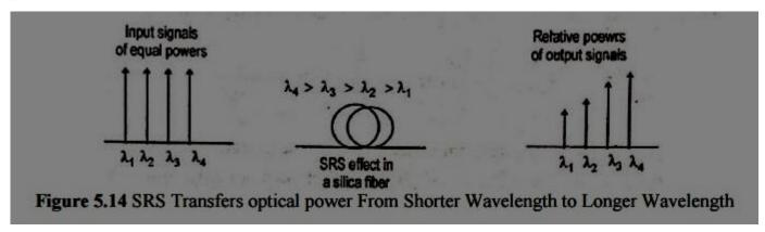
• COMMUNICATION SYSTEM by transferring energy from short-wavelength channels to
