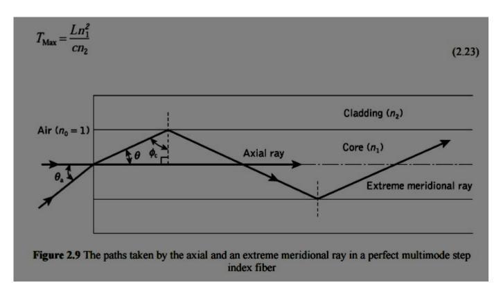
The delay difference  $\delta T$ s between the extreme meridional ray and the axial ray may be obtained by:
