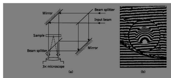
Figure 4.11 (a) The principle of the Mach–Zehnder interferometer. (b) The interference fringe pattern obtained with an interference microscope from a graded index fiber
