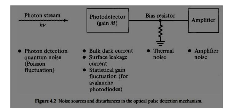
✓…Thermal noises arising from the detector load resistor and from the amplifier electronics tend to dominate in applications with low SNR when a PIN photodiode is used.
