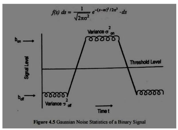
•□□□□□□□□□□□Now, we can use the probability density function to determine the probability of error for a data stream in which the 1 pulse are all of amplitude V.
