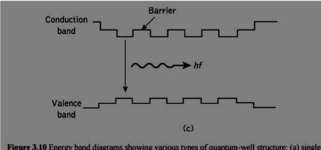
Figure 3.10 Energy band diagrams showing various types of quantum-well structure: (a) single quantum well; (b) multiquantum well; (c) modified multiquantum well
