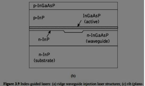
More typically, the threshold currents for such weakly index-guided structures are in the range 40 to 60 mA, which compares a light output versus current characteristic for a ridge waveguide laser with that of an oxide stripe gain-guided device. Alternatively, the application of a uniformly thick, planar active waveguide can be achieved through lateral variations in the confinement layer thickness or the refractive index. However,
