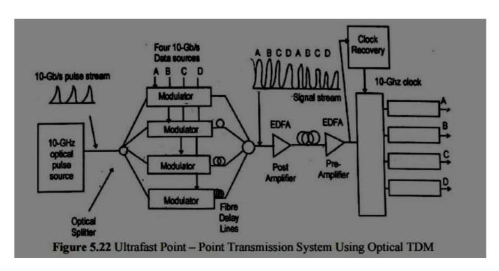
Repetition rate typically ranges from 2.5 to 10 Gb/S, which corresponds to the bit rate of the electric data tributaries feeding the system.
