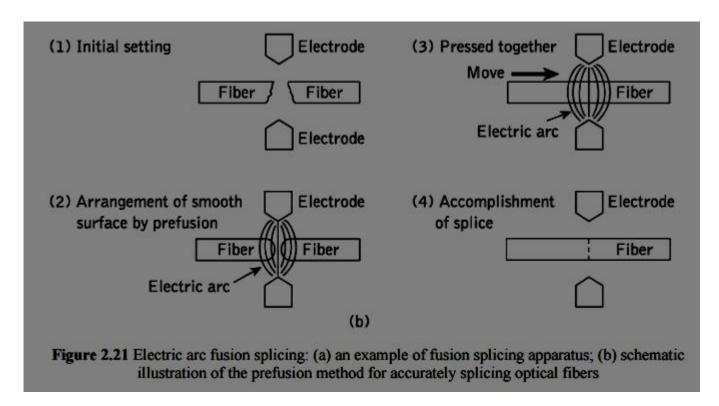
Fusion splicing of single-mode fibers with typical core diameters between 5 and 10  $\mu$ m presents problems of more critical fiber alignment (i.e. lateral offsets of less than 1  $\mu$ m are required for low loss joints). However, splice insertion losses below 0.3 dB may be achieved due to a self-alignment phenomenon which partially compensates for any lateral offset.
