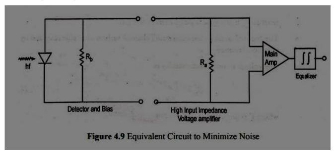
• □ □ □ □ □ □ □ □ □ □ □ □ It is compensated by differentiation in the equalizing fitter. This integration differentiation approach is known as the high impedance amplifier design technique.
