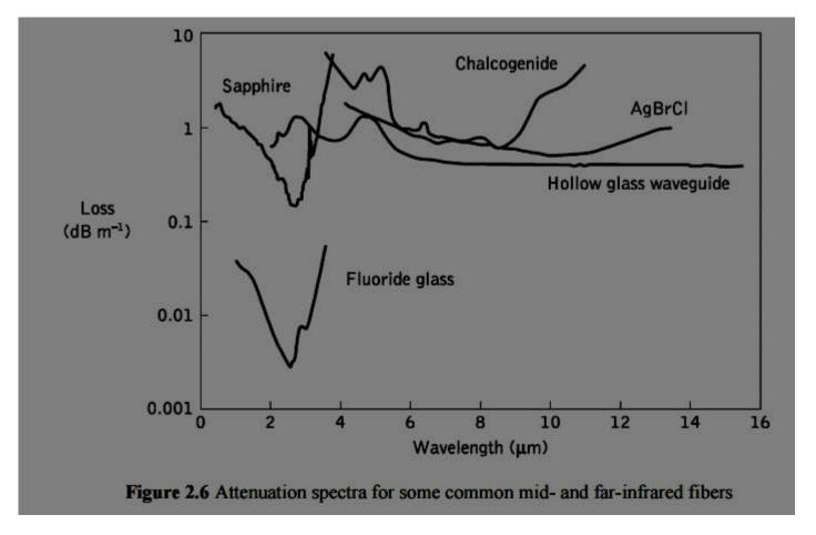
In particular, oxide glasses such as Al2O3 (i.e. sapphire) offer a near equivalent transmittance range to many of the fluoride glasses and have benefits of high melting points, chemical inertness, and the ability to be readily melted and grown in air. Chalcogenide glasses, which generally comprise one or more elements Ge, Si, As and Sb, are capable of optical transmission in both the mid-infrared and far-infrared regions.
