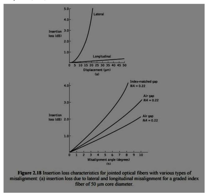
In this case there is still the problem of the quality of the fiber alignment provided by the jointing mechanism. Examples of possible misalignment between coupled compatible optical fibers are illustrated in Figure 2.17. It is apparent that misalignment may occur in three dimensions: the separation between the fibers (longitudinal misalignment), the offset perpendicular to the fiber core axes (lateral/radial/ axial misalignment) and the angle between the core axes (angular misalignment).
