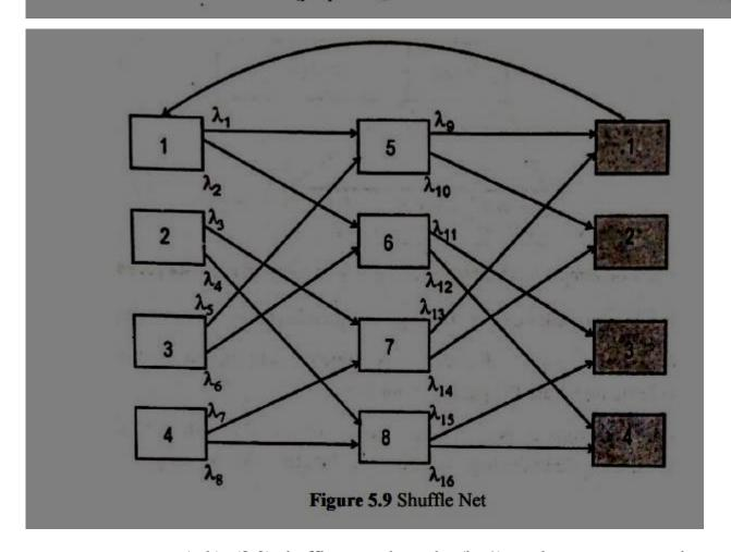
•  $\Box\Box\Box\Box\Box\Box\Box\Box\Box\Box\Box$  a (p,k)=(2,2) shuffle net, where the (k+1)th column represents the completion of a trip around the cylinder back to the first column.
