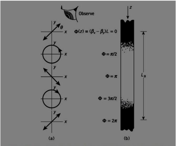
Figure 2.14 An illustration of the beat length in a single-mode optical fiber: (a) the polarization states against  $\Phi(z)$ ; (b) the light intensity distribution over the beat length within the fiber
