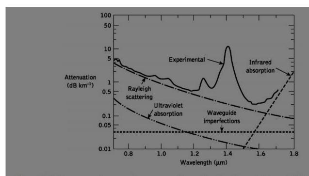
Figure 2.3 The measured attenuation spectrum for an ultra-low-loss single-mode fiber (solid line) with the calculated attenuation spectra for some of the loss mechanisms contributing to the overall fiber attenuation
