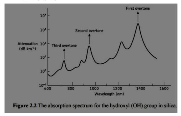
Furthermore, combinations between the overtones and the fundamental SiO2 vibration occur at 1.24, 1.13 and 0.88  $\mu$ m, completing the absorption spectrum shown in Figure 2.2.It may also be observed in Figure 3.2 that the only significant absorption band in the region below a wavelength of
