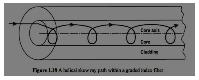
However, the near axial rays are transmitted through a region of higher refractive index and therefore travel with a lower velocity than the more extreme rays. This compensates for the shorter path lengths and reduces dispersion in the fiber. A similar situation exists
