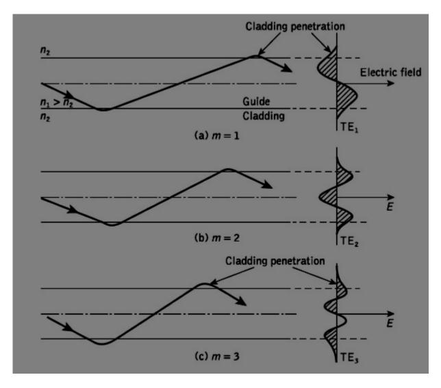
**Figure 1.9** Physical model showing the ray propagation and the corresponding transverse electric (TE) field patterns of three lower order models (m = 1, 2, 3) in the planar dielectric guide
