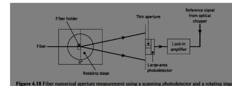
For the general case of a graded index fiber these local numerical apertures NA(r) at different radial distances r from the core axis may be defined by:
