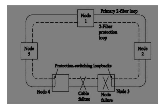
If both primary and secondary are cut, still the connection is not lost, but both the primary and secondary fibers of the entire ring is occupied
