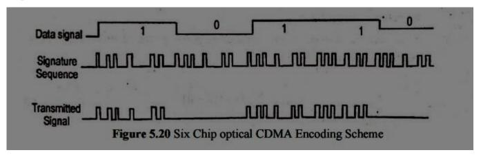
The signature sequence contains six chips. When the data signal contains 1 data bit, the six-chip sequence is transmitted, no chips are sent for a 0 data bit.
