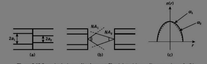
Figure 2.19 Some intrinsic coupling losses at fiber joints: (a) core diameter mismatch; (b) numerical aperture mismatch; (c) refractive index profile difference
