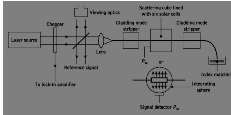
Figure 4.8 An experimental setup for measurement of fiber scattering loss illustrating both the solar cell cube and integrating sphere scattering cells
