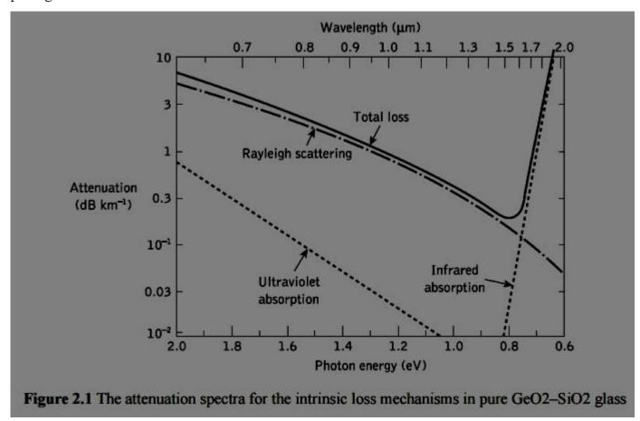
It may be observed that there is a fundamental absorption edge, the peaks of which are centered in the ultraviolet wavelength region. This is due to the stimulation of electron transitions within the glass by higher energy excitations.
