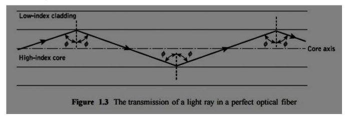
Figure 1.3 illustrates the transmission of a light ray in an optical fiber via a series of total internal reflections at the interface of the silica core and the slightly lower refractive index silica cladding. The ray has an angle of incidence  $\varphi$  at the interface which is greater than the critical angle and is reflected at the same angle to the normal.
