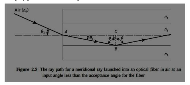
Assuming the entrance face at the fiber core to be normal to the axis, then considering the refraction at the air—core interface and using Snell's law given by Eq. (1.1):
