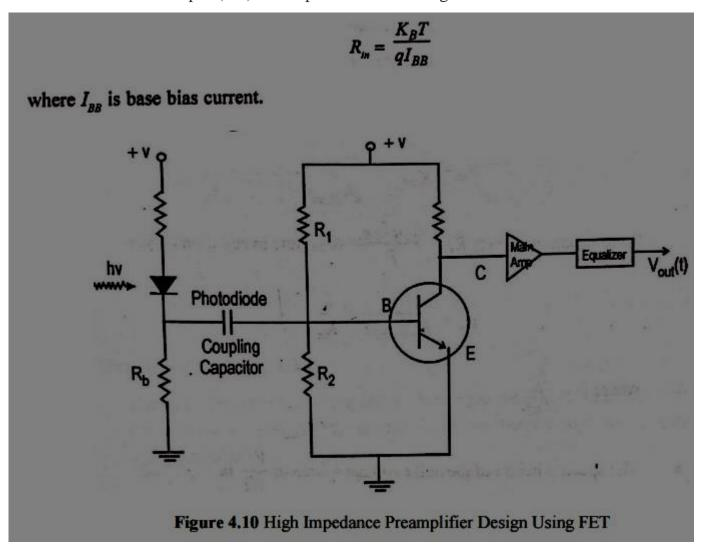
•  $\square$   $\square$   $\square$   $\square$   $\square$   $\square$   $\square$   $\square$   $\square$  The amplifier input resistance  $R_a$  is given by the parallel combination of the bias resistor  $R_1$  and  $R_2$  and the transistor input resistance  $R_{in}$ .
