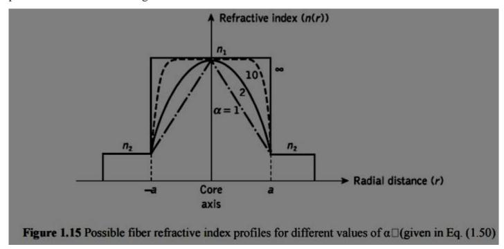
The graded index profiles which at present produce the best results for multimode optical propagation have a near parabolic refractive index profile core with  $\alpha \sim 2$ . Fibers with such core index profiles are well established and consequently when the term 'graded index' is used without qualification it usually refers to a fiber with this profile.
