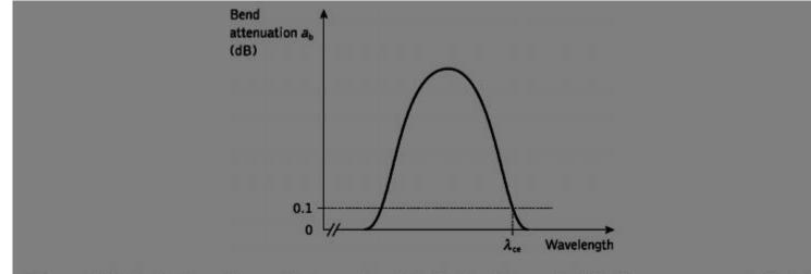
Figure 4.17 Bend attenuation against wavelength in the bending method for the measurement of cutoff wavelength λce
