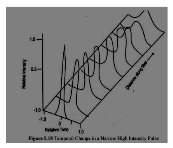
When a narrow high-intensity pulse traverse a medium with a negative GVD parameter for the constituting frequencies, GVD counteracts the chirp produced by SPM.
